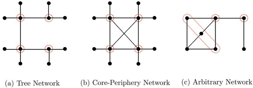
Figure 1: Example Networks with Disjoint Minimal Cut Sets
